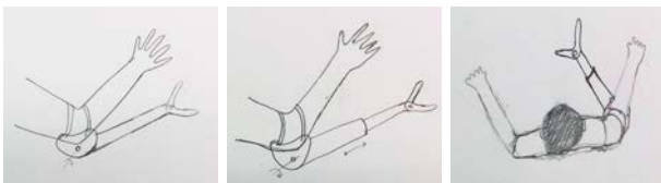
Fig. 4. Initial concept sketches for an elbow-mounted third arm robot (from left): a) Single vertical DoF, b) one vertical and one prismatic DoF, c) one horizontal and one prismatic DoF (chosen design).
