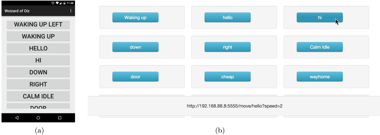
Figure 3: Mobile (a) and Dynamic HTML (b) OpenWoZ clients. A mouse hover in the HTML client shows the RESTful URI sent by the client to the HTTP Server.
